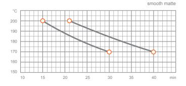
Please observe cure parameters closely since mechanical properties will develop before full cross-linking!
